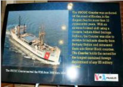
These, along with a pair of 35kW Collins short-wave units, were anchored off the coasts of certain communist states. Large helium barrage balloons hoisted long wire antennas and VoA was successfully heard in these countries over jamming interference.
