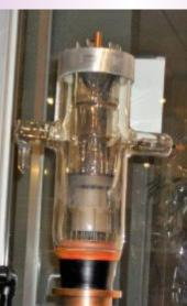
the immense size of this beast, this was one of the final tubes from **Powell Crosley** Jr's 500 kW AM transmitter. (WLW Cincinnati, circa 1930s.) There were 12 of these tubes in the final stage. Cooling water was pumped through the copper pipes in the base.
