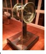
the device operated in the "bridge," tells the engine room chief the speed the captain wants to go. To add to the dramatic scene, the room where actual plates of the hull are hung, are chilled to the temperatures the passengers experienced
