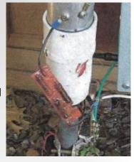
gested that 2 or 3 resistors in series should be installed. I took the idea a bit further. I now protect both vertical and long wire antennas, by using a small aluminum project box, Installing two SO-239's top and bottom, and installing one resistor from the center feed through conductor, to the box and shield ground.
