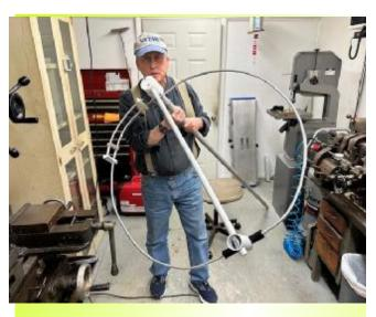
It is tuned with a gamma match using tubing that I had to cut precisely and adjust using my Nano-VNA. It is tuned close to the 6 Meter calling frequency of 50.125 MHZ and has fine SWR readings up to 51 MHZ, making it very narrow banded but good for the USB phone portion of the 6-Meter Band. However, the dimensions in the 25th AARL Antenna book article were different from the QST article it referenced in the 1975 QST article, so the Antenna was tuning to 147 MHZ, which was way out of band.
